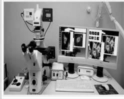
An experimental chamber (500 µl) with a suspension of cells was placed on the slide of an inverted microscope Axiovert 100M with a laser scanner LSM 5 (Zeiss, Oberkochen, Germany). Confocal images were obtained with a Zeissplan-Apochromat 40x1.4 lens. Visualization of changes [Ca<sup>2+</sup>], was performed using high-affinity (kd = 325 nM) Ca<sup>2+</sup> -sensitive fluorescent dye a Fluo-3 AM (максимуми абсорбції/емісії=506 нм/526 нм.
